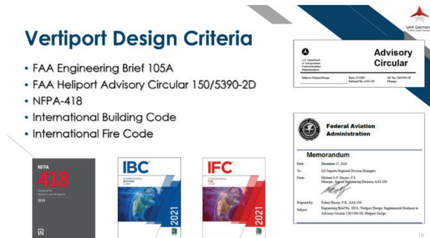
Figure 14 - These regulatory standards – FAA Engineering Brief 105A, FAA Heliport Advisory Circular 150/5390-2D, NFPA-418, the International Building Code, and the International Fire Code – must be applied in the design and development of the vertiport to ensure compliance, safety, and operational efficiency.
